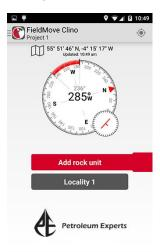
**Compass** face. The set bearing is shown by the red bar.
